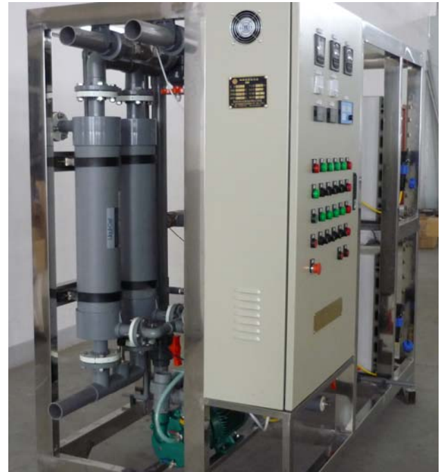
6-inch Liqui-Cel® Membrane Contactor System Upstream of EDI
